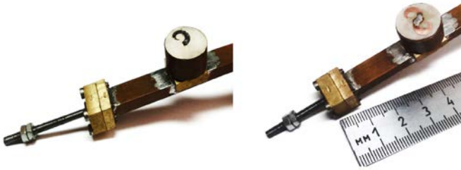
Fig.6 Two antenna prototypes: single planar spiral antenna (a); double (b)
